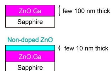
Figure 6 Schematic illustration of ZnO film prepared by MBE.
