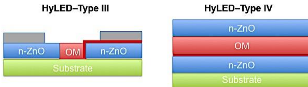
Figure 5: Injection HYLED-Type III and IV devices (description see text)
